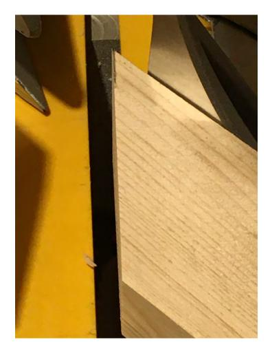
Helpful tip: Once the bars are cut to length place the boards that will be opposite one another back to back and compare their length. Each pair of boards must be the exact same length. If one is longer than the other mark the longer board with the shorter board and recut. You need 2 pairs of matching lengths to have a support with squared right angle corners.
