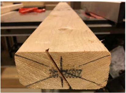
As you can see here, the cut is off center. This will result in uneven bars. Adjust the table saw's cutting fence to correct this.
