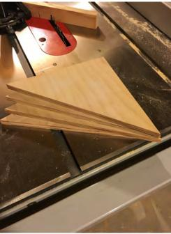
9- Slowly and carefully guide the board through the blade. Keep your fingers away from the blade and use a pus bar or push pads if you can. Repeat for the remaining squares of plywood. You only need 4 triangles for this project, but it is nice to make them in batches.
