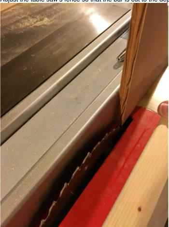
7- Cut the bar just to the previous cuts on the board. You should now have a recessed slot in the bar for the corner brace.
