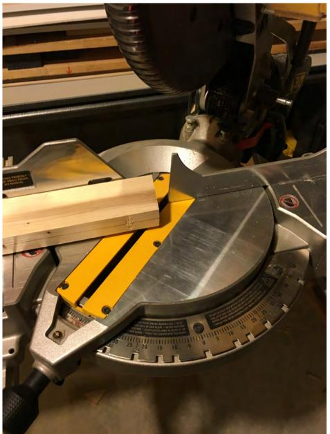
Note the angle of the miter cut. The lower side of the bar should also become the sorter side after the cut.
