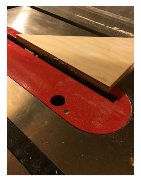
4- With the miter fence still set at 45° run each bar past the blade along the line you just marked. The blade should pass to the outside of the line closer to the end of the bar. You might want to use the table saw to "nibble" a little more of the wood away from the board by making a few more passes with the saw, each cut should be slightly closer to the end of the bar.
