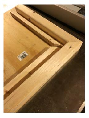
Helpful tip: this jig will be used to hold your corners at a 90° angle. If the jig isn't square your support will not be square. Take the time to make sure you are making a jig with a true right angle, and check it before you use it.
