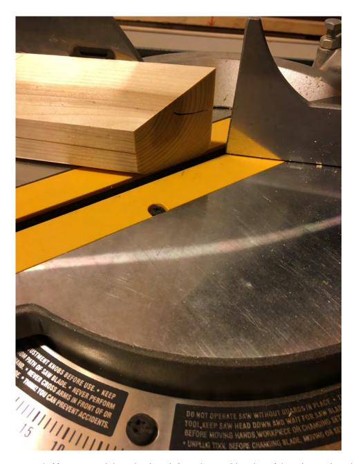
2- Measure each board to length from the outside edge of the miter and mark the length with a sharp pencil line. If you want the bar to be 60", as in this example, the longest edge of the bar needs to be 60". The inside length of the bevel will be shorter than 60"
