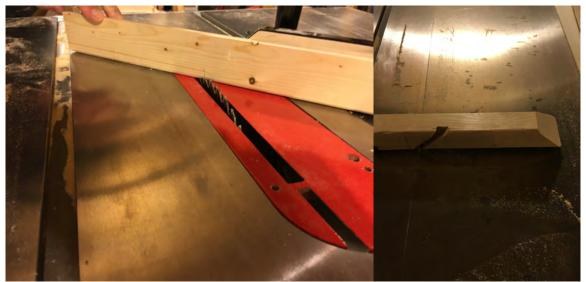
5- Use the plywood corner to mark the thickness of the plywood on the bar.
