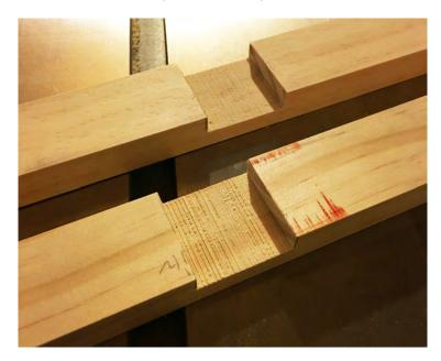
9- Attach the two braces to one another by placing one dado into the other. Use a small screw to attach the two pieces together at the joint. It is a good idea to pre drill the hole since this material is a bit thin.
