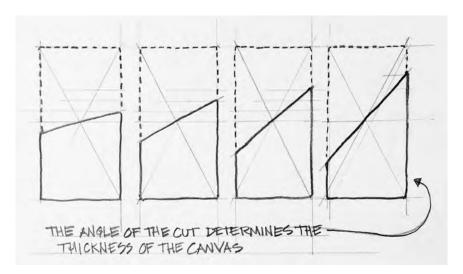
3- Set up the table saw by lifting the blade and tilting it to  $30^{\circ}$ . Male sure the blade is elevated just high enough to cut completely through the 2 x 4. Make sure the blade tilts away from the table saw's fence.
